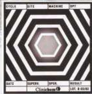
Air pocket (light spot in or near the centre of the sheet)
