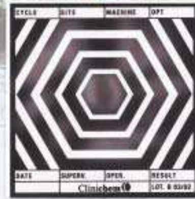
Wet steam or non condensable gases (spots/figures/circle formed figure in the center)
